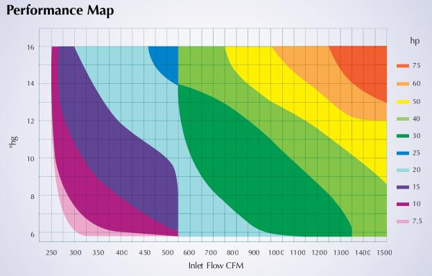
Performance based on inlet air at standard temperature of 68°F, an ambient pressure of 14.7 psia and 36% relative humidity. For performance at non-standard conditions, contact your authorized AVI representative.
